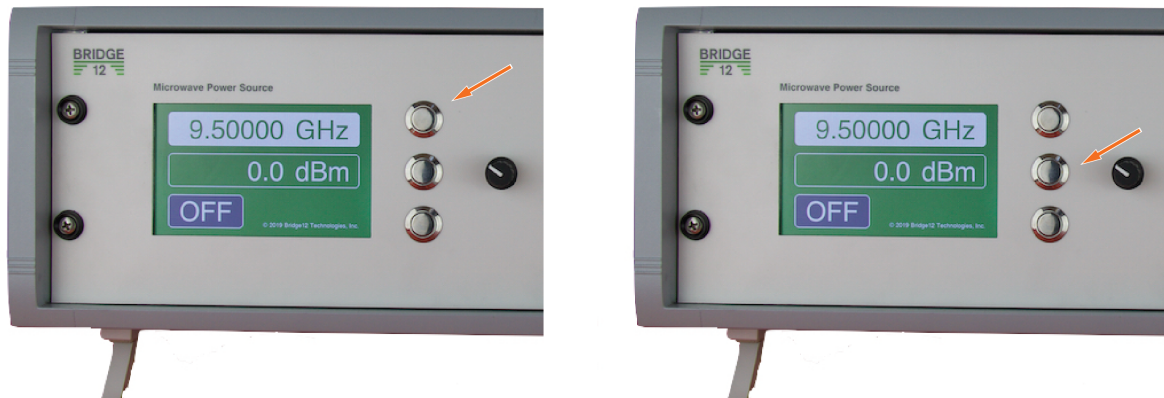
Figure 5.1: Left: MPS set to change the output frequency. Right: MPS set to change the output power level
