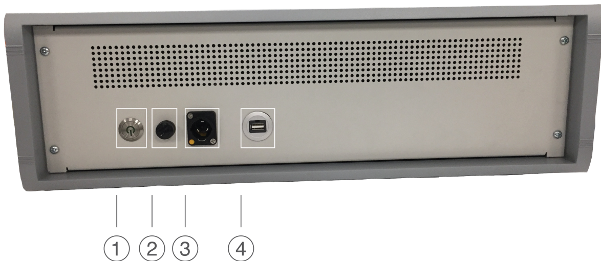
Figure 1.2: Bridge12 MPS Back Panel
