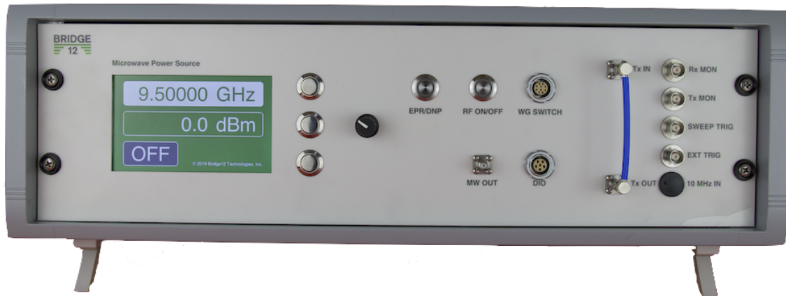
Figure 4.4: Front panel display of main screen. The system is ready.
