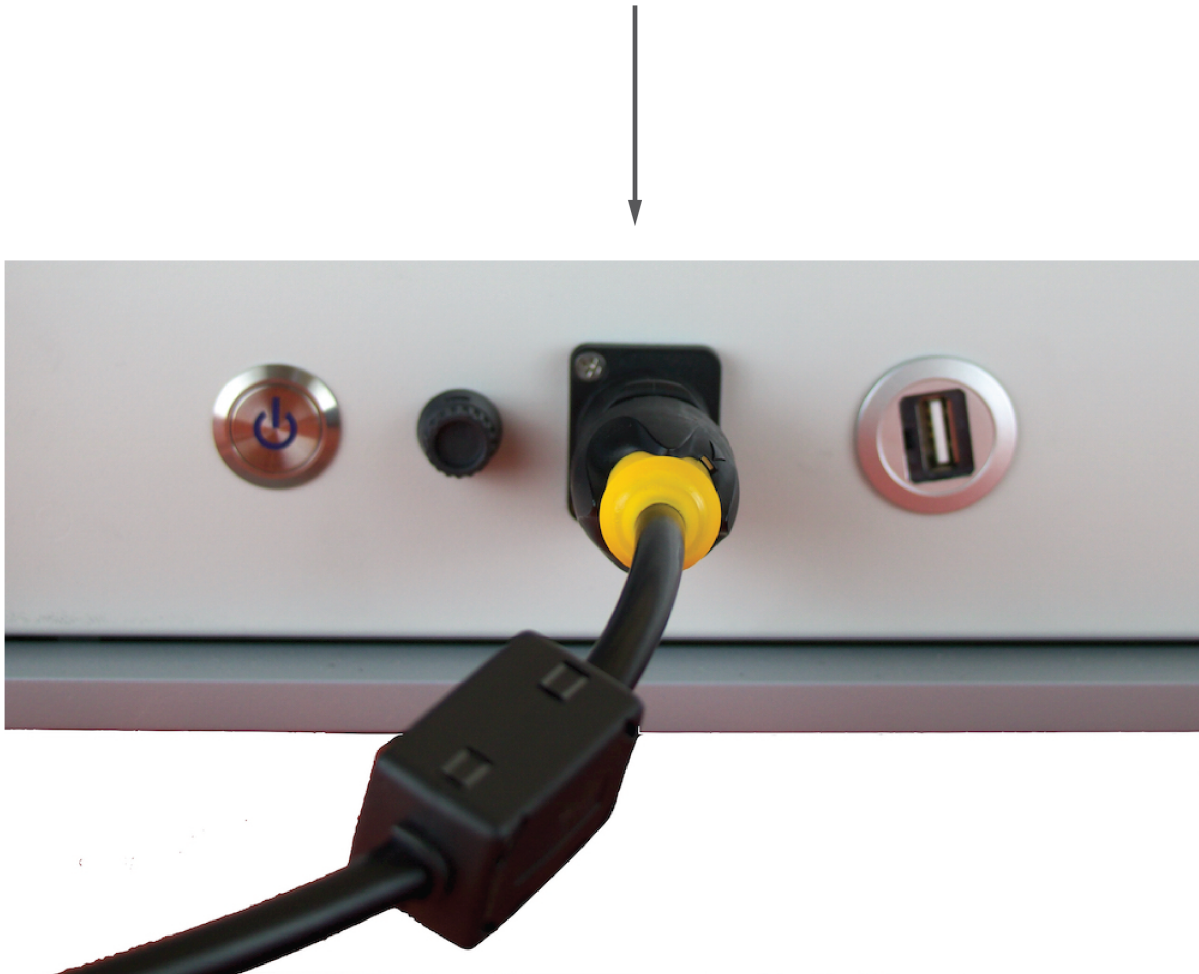
Figure 4.1: Back panel power connector
