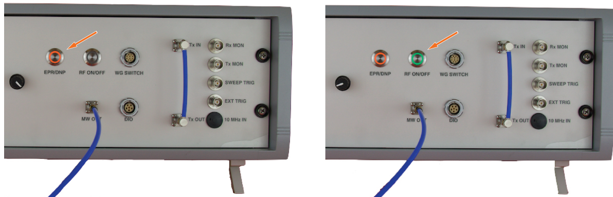
Figure 5.2: Left: Waveguide switch control button (orange). Right: Microwave (RF) ON/OFF button (green)
